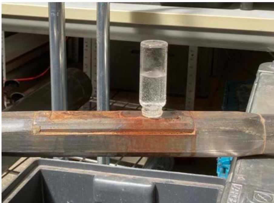
Figure 2: MIP probe with sample during measurement
